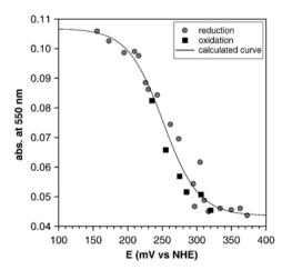
Fig. 6. Redox titration of the  $c_{552}$  (4  $\mu$ M, pH 6.6) showing absorption at 550 nm (from ferrous cytochrome) as a function of solution potential. The solid line shows the Nernstian curve for a single electron transfer at a potential of  $+251\pm5$  mV vs. NHE. The reductive and oxidative directions of the titration are indicated by circles and squares respectively. See Materials and methods for other conditions.
