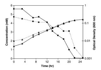
Fig. 3. Growth of NT-26 and NT-26 *cytC* mutant in a minimal salts medium containing arsenite (5 mM) and yeast extract (0.04%). NT-26 wild-type, solid lines and NT-26 *cytC* mutant, dashed lines. Arithmetic plot: ■, concentration of arsenite. Logarithmic plot: ▲, optical density.
