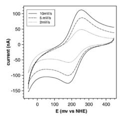
Fig. 7. Cyclic voltammograms of  $c_{552}$  (20  $\mu$ M) at sweep rates of 2, 5 and 10 mV s<sup>-1</sup> (pH 7.1). See Materials and methods for other conditions. The averaged potential of the reductive (negative) and oxidative (positive) peaks is +217 mV vs. NHE.
